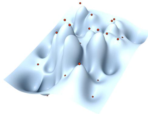
The first iteration started with a flat surface, with all the normals pointing directly upwards. However, after the control-points were adjusted, the surface is far from planar. Since we restrict Control Point motion along the normal of the Greville Point, the surface now starts to bulge horizontally as well. Deviation reduced to 34mm.
