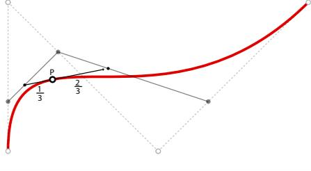
One final iteration gets rid of the last line segment and we are left with point {P}, which is ON the spline, at parameter  $1/3$ .
