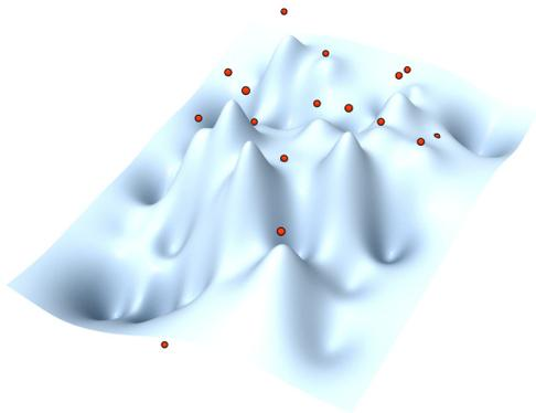
This image is recognizable as a 3D version of the diagrams you've seen before. Every point has a small summit pointing towards it. This is the result of the first iteration of our algorithm. Total deviation is still 63mm (measured as total distance between all red points and their projection onto the surface).
