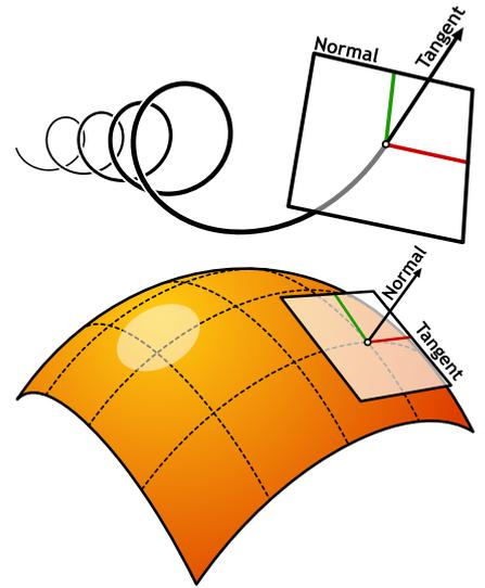
In the case of NURBS surfaces there are in fact two directions implied by the geometry, because NURBS surfaces are rectangular grids of  $\{u\}$  and  $\{v\}$  curves. And even though these directions are often arbitrary, we end up using them anyway because they make life so much easier for us.
