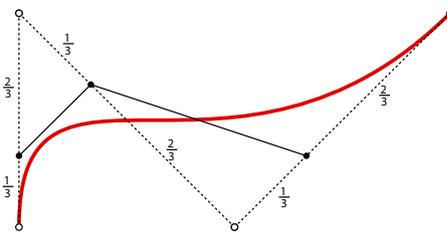
Let us say we want to find the Point {P} which is one third of the way between {A} and {D}. Note that this is not a third of the *distance* along the spline, but a third of the parameter domain. A curve like this has a parameter domain from 0.0 to 1.0, regardless of its actual dimensions.
