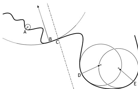
Points {A; B; C; D; E} have a certain curvature associated with them. The radius of the respective circles is a measure for the curvature (in fact, the curvature is the inverse of the radius), and the direction of the vectors is an indication of the curve plane.
