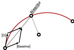
The halfway point on the arc *also* happens to lie on the bisector between {D} and the baseline vector. We can easily construct the bisector of two vectors in 3D space by process of unitizing and adding both vectors. In the illustration on the left the bisector is already pointing in the right direction, but it still hasn't got the correct length.
