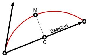
We're going to find the coordinates of the point in the middle of the desired arc {M}, so we can use the 3Point approach with {A}, {B} and {M}. As the illustration on the left indicates, the point in the middle of the arc is also on the line perpendicular from the middle {C} of the baseline.
