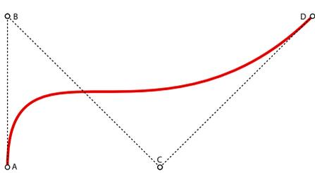
On the left you see a standard (cubic) Bézier curve. The curve begins at {A} and ends at {D}. The direction of the vectors {AB} and {DC} control the tangents at the end points.
