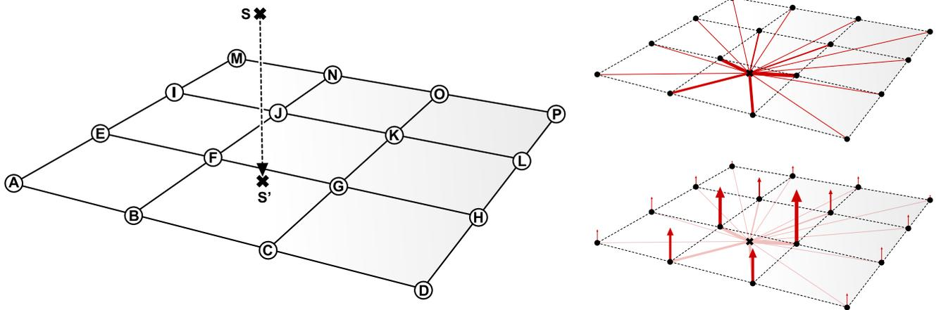
For purposes of clarity I have unfolded a very twisted nurbs patch so that it is reduced to a rectangular grid of control-points. The diagram you're looking at is drawn in  $\{uvw\}$  space rather than world  $\{xyz\}$  space. The actual surface might be contorted in any number of ways, but we're only interested in the simplified  $\{uvw\}$  space.
