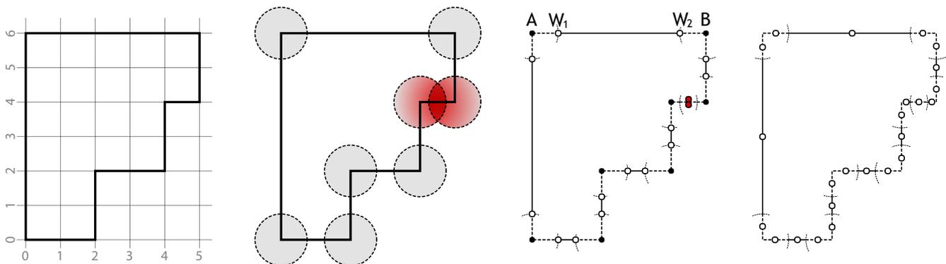
The first image shows our input curve positioned on a unit grid. The shortest segment has a length of 1.0, the longest segment a length of 6.0. If we're going to blend all corners with a radius of 0.75 (the circles in the second image) we can see that one of the edges has a conflict of overlapping blend radii.
