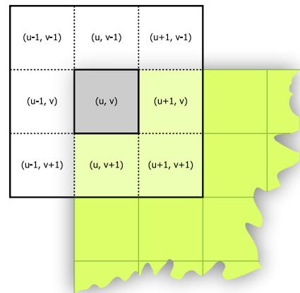
The green area is a corner of the entire two-dimensional tensor space, the dark green lines delineating each individual tensor. The dark grey square is the tensor we're currently working on. It is located at {u,v}. The eight white squares around it are the adjacent tensors which will be used to blur the tensor at {u,v}.
