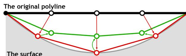
The illustration depicts the two steps which compose a single iteration of the geodesic routine. The black polyline is projected onto the surface giving the red polyline. The red curve in turn is smoothed into the green curve. Note that the actual algorithm performs these two steps in the reverse order; smoothing first, projection second.
