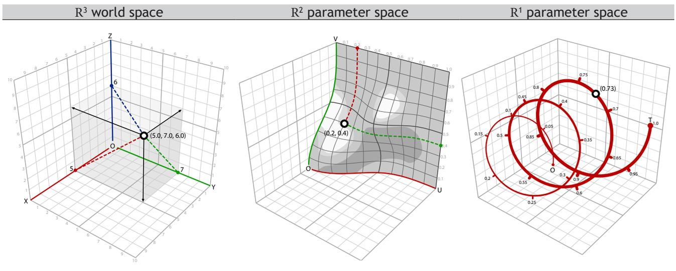
The image on the left shows the  $R^3$  world space, it is continuous and infinite. The x-coordinate of a point in this space is the projection (the red dotted line) of that point onto the x-axis (the red solid line). Points are always specified in world coordinates in Rhino.
