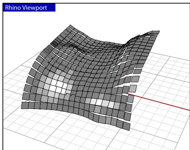
The `rs.SurfaceFrame()` method returns a unitized frame whose axes point in the [u] and [v] directions of the surface. Note that the [u] and [v] directions are not necessarily perpendicular to each other, but we only add valid planes whose x and y axis are always at 90°, thus we ignore the direction of the v-component.
