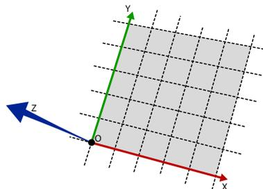
A plane definition is an array of one point and three vectors, the point marks the origin of the plane and the vectors represent the three axes. There are some rules to plane definitions, i.e. not every combination of points and vectors is a valid plane. If you create a plane using one of the RhinoScript plane methods you don't have to worry about this, since all the bookkeeping will be done for you. The rules are as follows:
