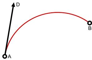
We start with two points {A} & {B} and a vector definition {D}. The arc we're after is the red curve, but at this point we don't know how to get there yet. Note that this problem might not have a solution if {D} is parallel or anti-parallel to the line from {A} to {B}. If you try to draw an arc like that in Rhino it will not work. Thus, we need to add some code to our function that aborts when we're confronted with unsolvable input.
