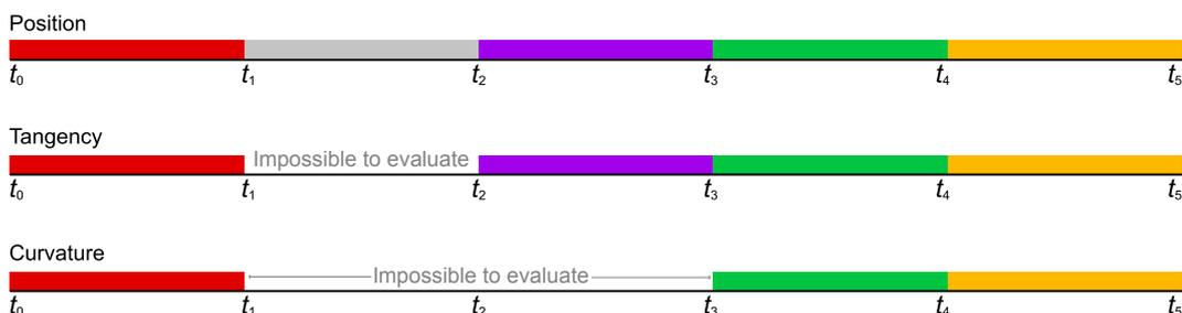
When using curve properties such as tangents, curvature or perp-frames, we must always be careful to not blindly march on without checking for property discontinuities. An example of an algorithm that has to deal with this would be the `_CurvatureGraph` in Rhino. It works on all curve types, which means it must be able to detect and ignore linear and zero-length segments that lack curvature.
